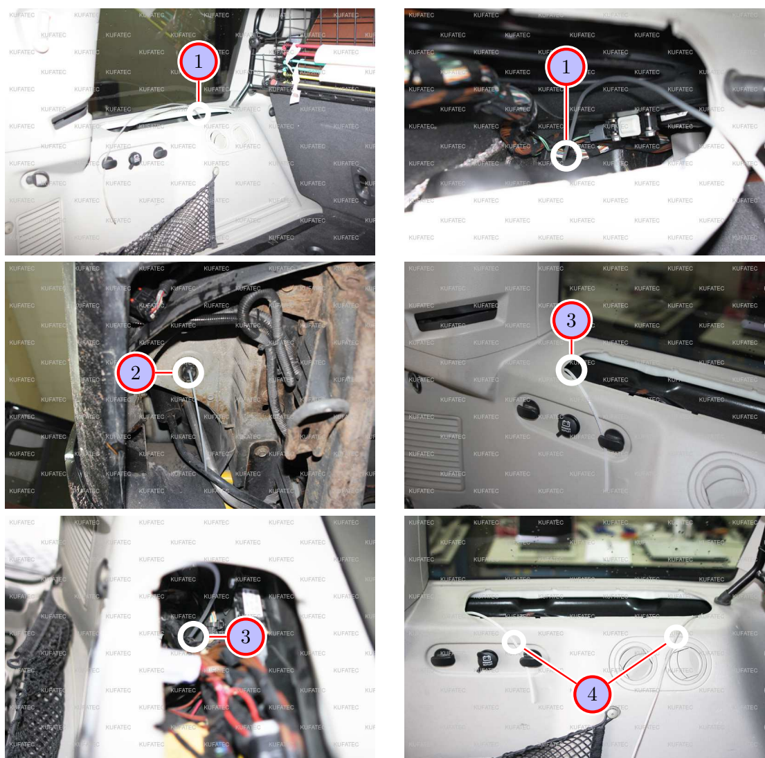
Figure 8: Cable routing to the underbody
