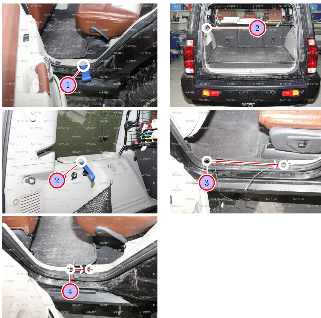
Figure 7: Cable routing to the trunk
